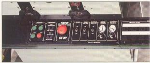
**Master control:** The master control was designed with in streamlined panel. Included are (from left to right): all dieclistration controls, run controls, rewind controls, and sheete allows the operator the greatest function and convenience
