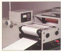
Tension control: A load cell monitoring system is the most sophisticated method for controlling web tension. It measures tension as the web passes over its surface, feeding the information electronically to the unwind brake, where minute adjustments are
